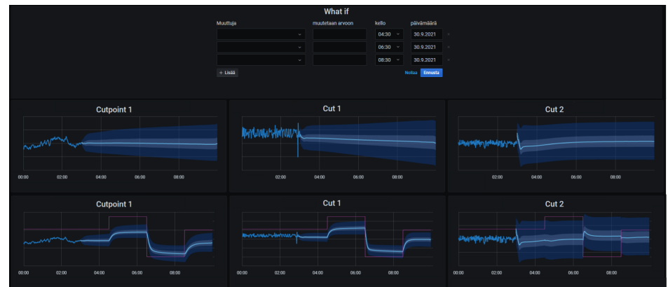
Example of a what-if scenario produced by NAPCON Advisor. Upper trend windows show normal predictions and lower trend windows show the effect of the implemented what-if scenario.
