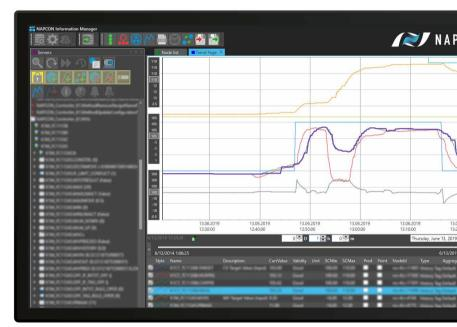
Trend views offer a convenient way to monitor control performance. Versatile trending options are available for control performance and controller parameters.
