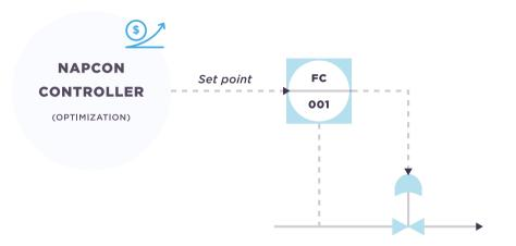
NAPCON Controller calculates new optimal set point values for basic controllers on each control cycle. The objective is to push the process to the best operating point as defined by advanced process control targets and constraints. The cycle length is adjustable from a few seconds to several minutes.
