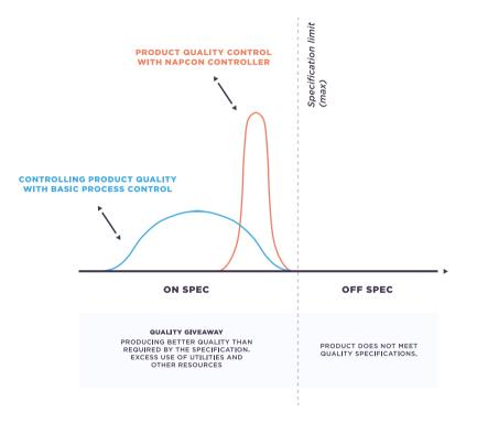
The optimal process operation is to run as close as possible to the process limits. NAPCON Controller decreases variance in main quality variables and keeps the process safely and economically near, but on the right side of the constraints.
