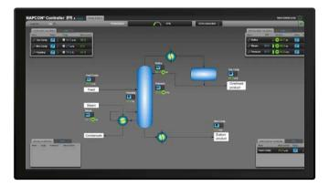
NAPCON Controller operator user interface is based on the web technologies. It can be seamlessly integrated to all modern DCS or SCADA operating environments and facilitates fluent workflow for panel operators.
