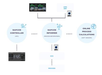
OPC UA communication is used between NAPCON applications. That offers seamless integration between NAPCON Controller APC algorithm and online process calculations providing data for advanced process control.
