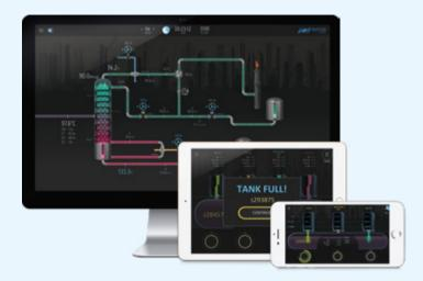
The competition included a multicomponent distillation column simulation and the player had to find out whether a stream will fit into a certain point. The highest and lowest concentration of the distillation column in regards to key components could be viewed by the player.
