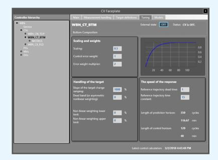
NAPCON Controller faceplates provide access to full spectrum of control parameters for best control performance.
