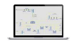
NAPCON Lite OTS is a generic level simulator that offers a possibility to train plant personnel on particular technology or on a process without going to the specific process plant details.
